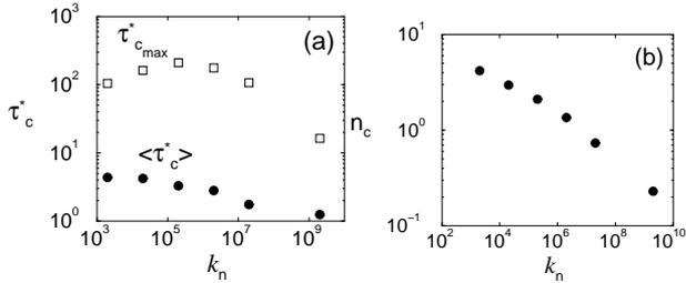
FIG. 3: Dependence on the particle stiffness  $k_n$ , of, (a) the depth-averaged contact lifetime  $\langle \tau_c^* \rangle$  (filled circles) and maximum contact time  $\tau_{c_{\max}}^*$  (open squares), both normalized by  $t_{\text{col}}$ , and (b) the depth-averaged number of contact neighbors per particle,  $n_c$ . Flow at  $\theta = 23^\circ$ .
