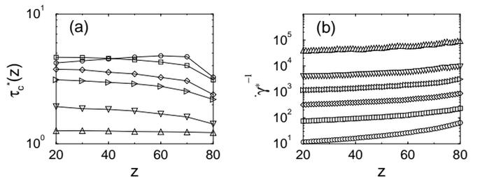
FIG. 2: Depth profiles of, (a) the normalized contact time  $\tau_c^*$  (line is a guide to the eye) and, (b) the normalized shear time  $\dot{\gamma}^{*-1} \equiv \dot{\gamma}^{-1}/t_{\text{col}}$ , for different particle stiffness,  $k_n = 2 \times [10^9 (\Delta), 10^7 (\nabla), 10^6 (\triangleright), 10^5 (\diamond), 10^4 (\square), 10^3 (\circ)] \text{ mg/d}$ .  $z = 0$  defines the bottom of the pile. Flow at  $\theta = 23^\circ$ .
