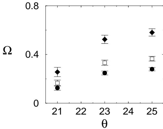
FIG. 5: Dependence of  $\Omega$ , on inclination angle  $\theta$ , at different heights inside the pile ( $h$ =top of pile):  $\frac{h}{4}$  (●),  $\frac{h}{2}$  (□), and  $\frac{3h}{4}$  (◆) for steady state flow for  $k_n = 2 \times 10^4 mg/d$ .
