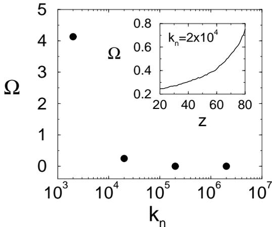
FIG. 4: Dependence of the parameter  $\Omega$  on the stiffness  $k_n$  for  $\theta = 23^\circ$ . Taken from the middle of the pile at  $h/2$ . Inset: Height dependence of  $\Omega$ , for  $k_n = 2 \times 10^4$ .
