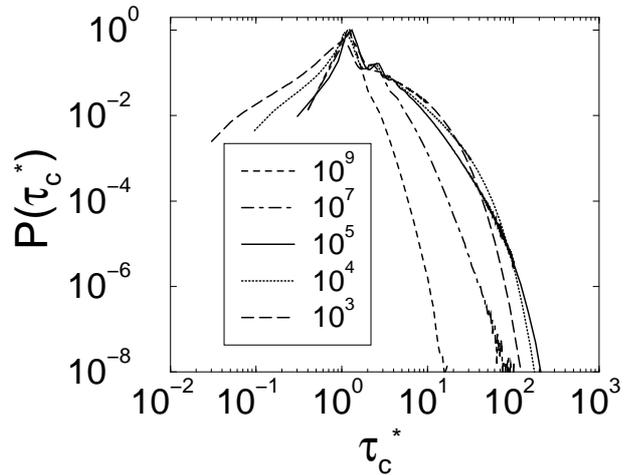
FIG. 1: Dependence of the distributions  $P(\tau_c^*)$  of the depth-averaged normalized contact lifetimes,  $\tau_c^* \equiv \tau_c/t_{\text{col}}$ , on particle stiffness  $k_n = 2 \times [10^9, 10^7, 10^5, 10^4, 10^3] \text{ mg/d}$ . Flow at  $\theta = 23^\circ$ .
