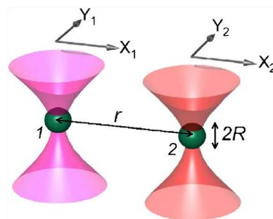
FIG. 1. (Color online) Schematic sketch of the two-particle microrheology experiment. A pair of silica particles (radius  $R$ ) is trapped by a pair of laser traps at a separation distance  $r$ . The position fluctuations of each particle in the  $x$  and  $y$  directions are simultaneously detected with quadrant photodiodes. The cross-correlated position fluctuations are measured parallel and perpendicular to the line connecting the centers of the particles.
