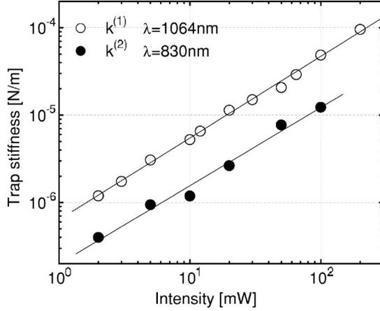
FIG. 3. Trap stiffnesses of two laser traps generated by independent lasers ( $\lambda = 1064$  and  $830$  nm) measured from the fluctuations of two silica particles ( $R = 0.58 \mu\text{m}$ ) in water. The trap stiffnesses increased linearly with the laser intensities (measured before the beams entered the objective) for both traps.
