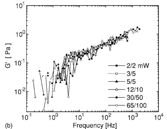
FIG. 13. Storage shear modulus of a 10 mg/ml *fd* solution as a function of frequency  $G'$ , measured with 2PMR in parallel direction. The trap powers were varied in parallel (measured before the objective, legend: 1064/830 nm powers), with the (a) *uncorrected* modulus  $G'$  and (b) the *actual* modulus  $G'$  calculated using the corrected response functions in Eq. (7c).
