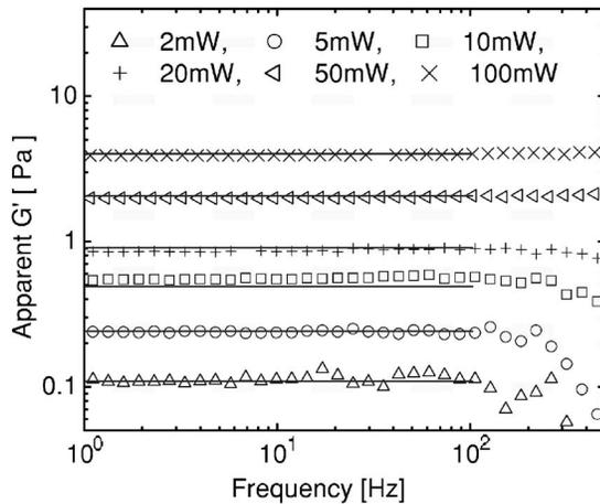
FIG. 5. Apparent storage moduli (caused by the trap) as a function of frequency, measured in water with IPMR for different laser powers (measured before the objective, see text). The solid lines are the theoretical predictions based on the measured trap stiffnesses.
