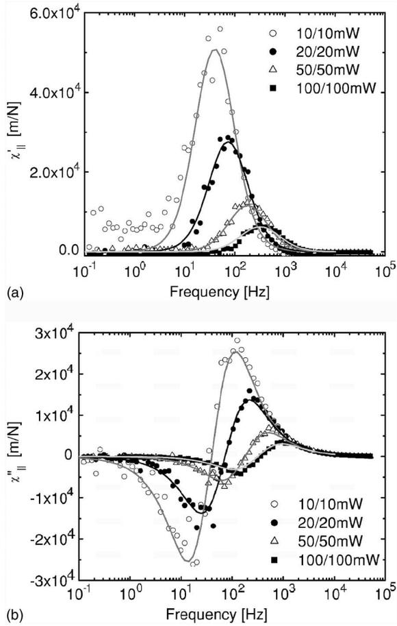
FIG. 10. (a) Real part and (b) imaginary part of the inter-particles response functions of two particles in water as a function of frequency,  $f = \omega/2\pi$  in the parallel direction, trapped with different laser powers varied in parallel in the two traps (measured before the objective, legend: 1064/830 nm powers). The theoretical predictions of Eq. (6c), calculated with the trap stiffness determined from corner frequency are plotted for comparison (lines).
