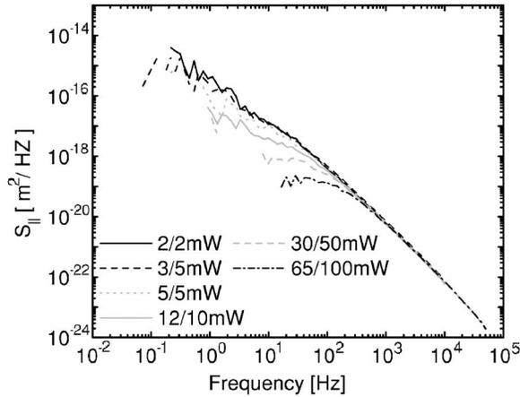
FIG. 12. Inter-particle correlation functions in the parallel direction of two particles separated by a distance  $r=2.9 \mu\text{m}$  in a 10 mg/ml *fd* solution, as a function of frequency. The trap powers were varied in parallel (measured before the objective, legend: 1064/830 nm powers). A power-dependent anticorrelation is observed at low frequencies.
