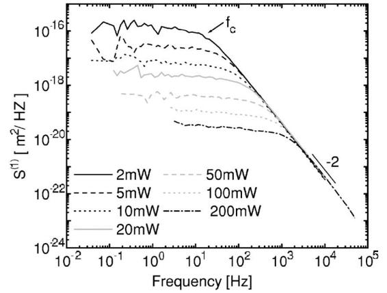
FIG. 2. Displacement autocorrelations of a particle trapped in water as a function of frequency  $f=\omega/2\pi$ . The laser intensity (wavelength  $\lambda=1064 \text{ nm}$ ) was varied between 3 and 150 mW. The corner frequency  $f_c$  changes with laser intensity; the high frequency power-law slope is  $-2$ . Laser noise (increasingly prominent for stronger confinement at higher powers) was cut off at the low-frequency end of the curves.
